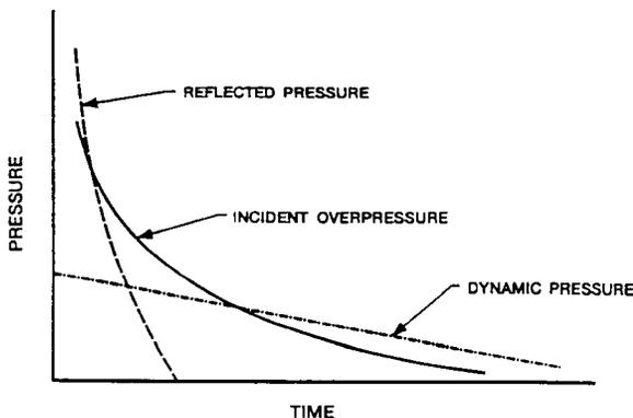
FIG. 2. Blast Wave Characteristics Related to Structural Loadings
